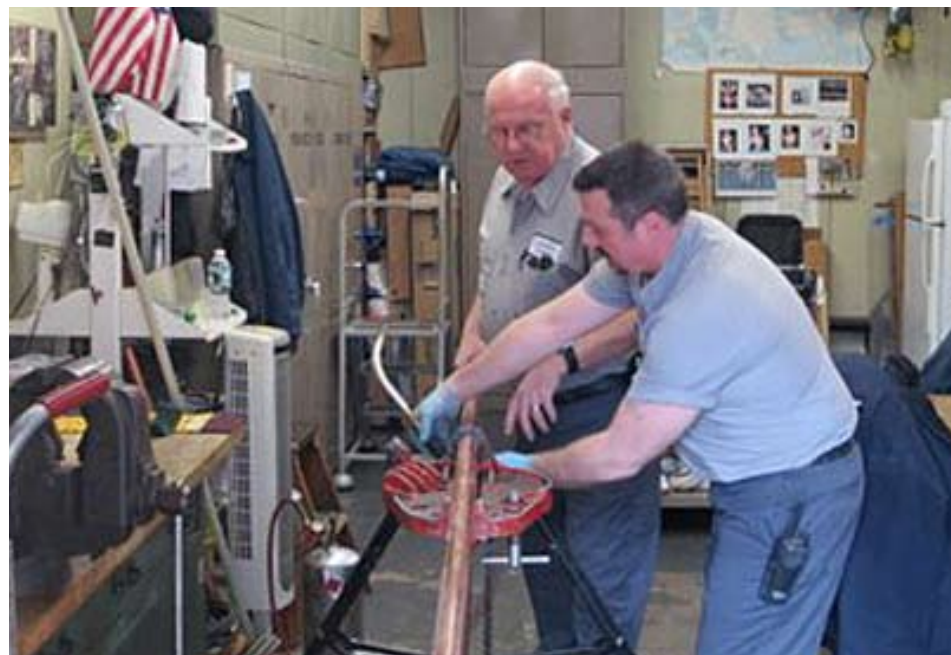
Mechanic Tom Brino (foreground) and Joe Janczewski cut some piping as part of an air conditioner repair.
